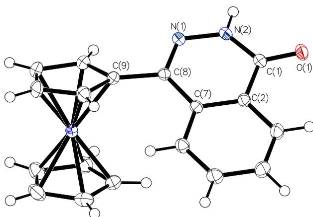
Fig. 2. Molecular structure of complex **V**. The most important bond length (Å): O1-C1 1.244(1), N2-N1 1.366(1), N2-C1 1.355(1), N1-C8 1.310(1), C7-C8 1.455(1), C7-C2 1.405(2), C8-C9 1.477(2) C2-C1 1.459(1).
