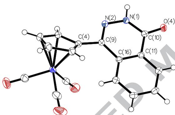
Fig. 3. Molecular structure of complex **VI**. The most important bond length (Å): O4-C10 1.245(2), N2-N1 1.364(2), N2-C9 1.300(2), N1-C10 1.363(2), C16-C9 1.457(2) C16-C11 1.409(2), C10-C11 1.456(2), C9-C4 1.479(2)
