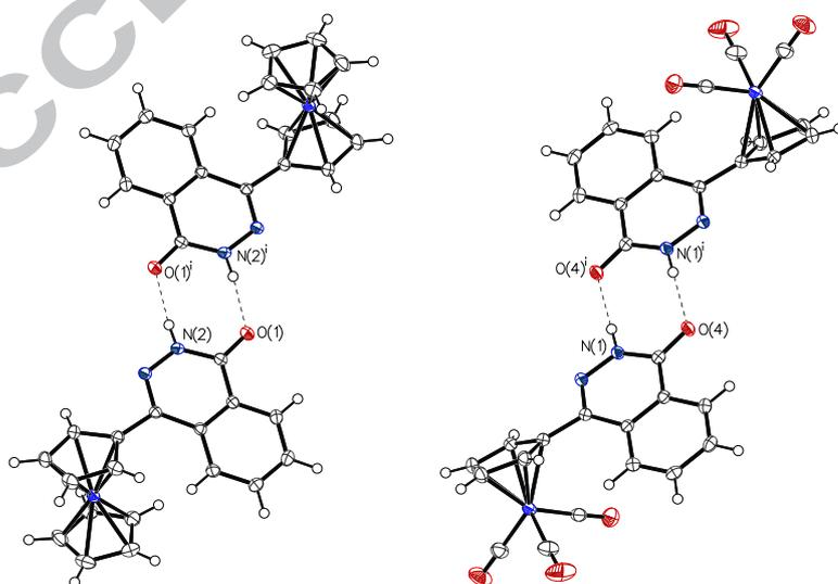
Fig. 4. Intermolecular double hydrogen bonds in phthalazine dimers **V** (N(2)-O(1)<sup>i</sup> 2.810(1) Å) and **VI** (N(1)-O(4)<sup>i</sup> 2.820(2) Å).
