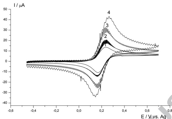
Fig. 6. CVs of complex **V** ( $C= 3.2$  mM) recorded at the GC electrode SU -2000 ( $0.0078$  cm<sup>2</sup>) in dichloromethane deaerated by high-purity argon with  $0.2$  M  $Bu_4NPF_6$  as the supporting electrolyte) in interval potentials  $(-0.45 \div 0.7)$  V with a different sweep rate,  $V s^{-1}$ : 1- 0.1; 2- 0.2; 3-0.5; 4- 1.0.
