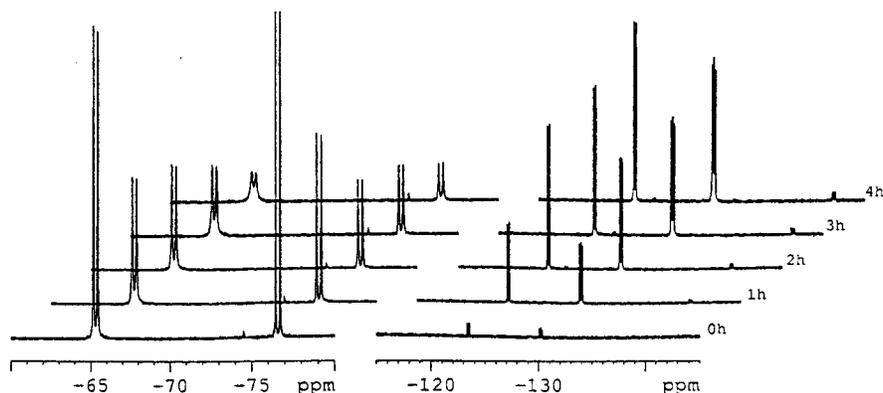
**Figure 4.** The  $^{19}\text{F}$  NMR spectra of the reaction mixture containing E 4-P, a 60:40 mixture of (*Z*)- and (*E*)-[3-F]-PEP and manganese(II) chloride in BTP buffer (pH 6.8) and 10%  $\text{D}_2\text{O}$  at various time intervals after addition of DAH 7-P synthase at room temperature. Chemical shifts of (*Z*)- and (*E*)-[3-F]-PEP are different from those in Figure 2 due to the presence of the buffers and the difference in the pH.
