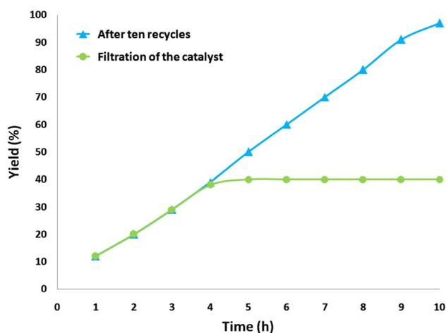
**Fig. 12** Leaching test for catalyst for synthesis of  $\beta$ -oxopropylcarbamate
