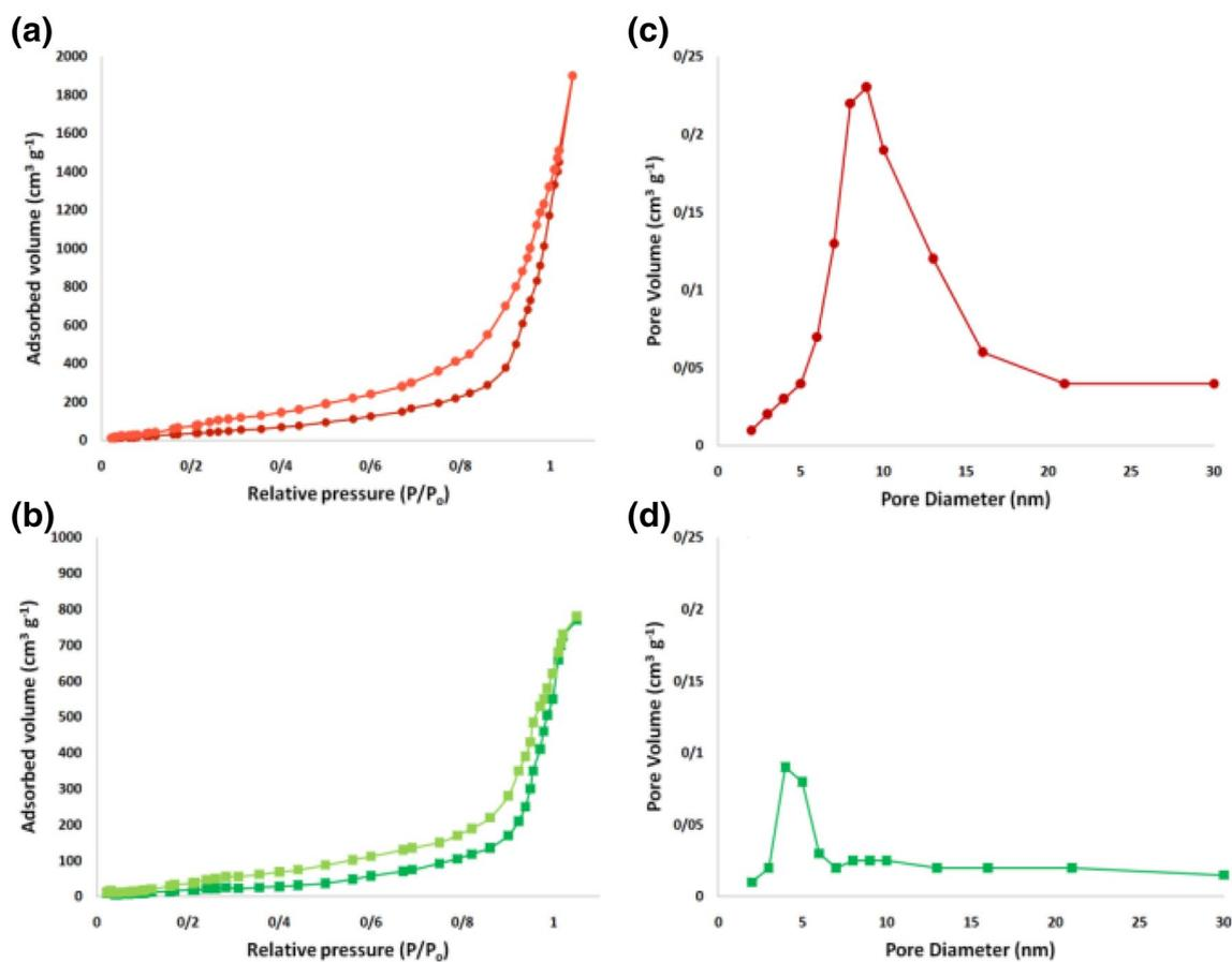
**Fig. 6** Adsorption–Desorption isotherms of the FPS NPs (a); TEMPO@FPS-laccase NPs (b); and BJH pore size distributions of the FPS NPs (c); TEMPO@FPS-laccase NPs (d)
