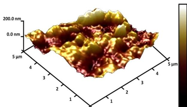
**Fig. 4** Three-dimensional of AFM images of TEMPO@FPS-laccase NPs
