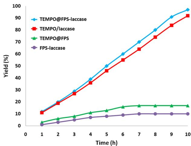
**Fig. 9** Synthesis of  $\beta$ -oxopropylcarbamate by different FPS nanoparticles
