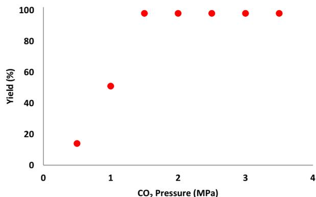
**Fig. 7** The effect of  $\text{CO}_2$  pressure on the synthesis of  $\beta$ -oxopropylcarbamate
