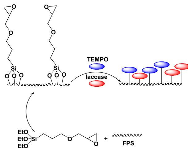
**Scheme 2** The process of co-immobilization of laccase and TEMPO onto glycidyoxypropyl-functionalized FPS nanoparticles
