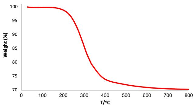
**Fig. 2** TGA diagram of TEMPO@FPS-laccase NPs
