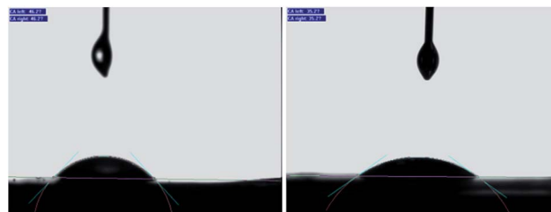
Fig. 4 Static contact angle measurement on separator with different electrolytes, without addition of DSGC (left) and with addition of DSGC (right).
