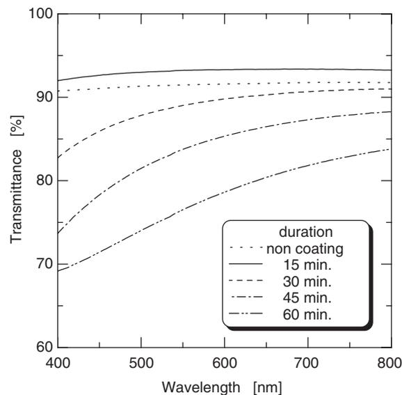
Fig. 2. Transmittances of visible light for variable hydrolysis reaction durations.
