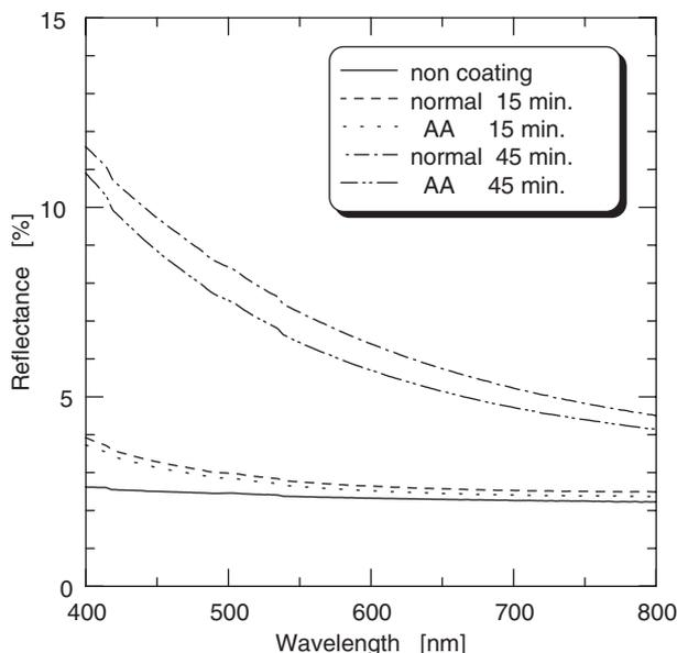
Fig. 7. Reflectances of visible light in the case with acetylacetone (AA).
