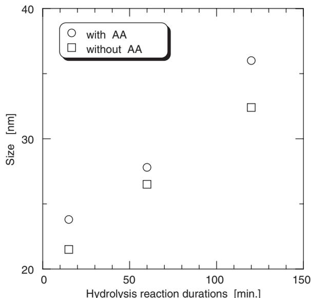
Fig. 8. Differences of particle size deposited on slide glass surface on addition of acetylacetone (AA).
