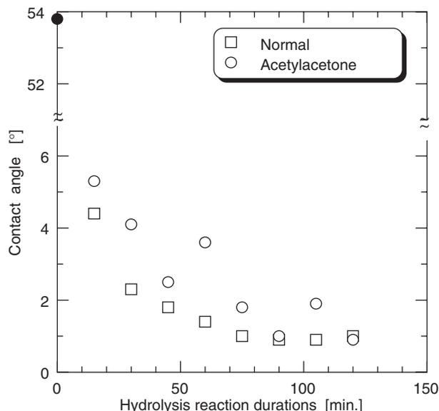
Fig. 6. Influence of addition of acetylacetone on contact angles of water.
