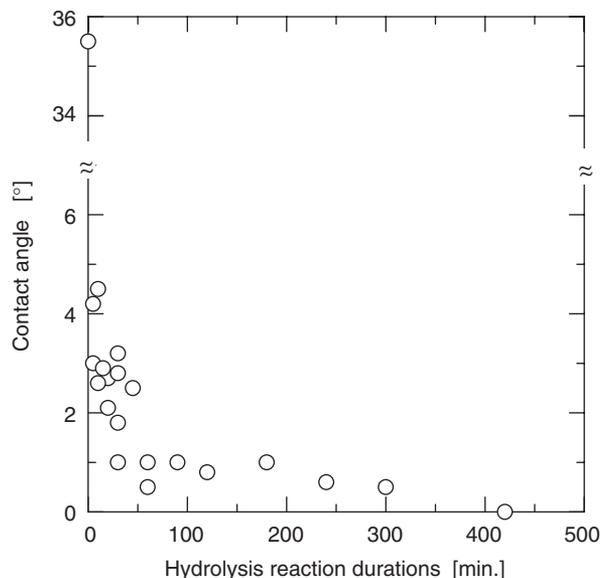
Fig. 1. Changes in contact angles of water with hydrolysis reaction duration.
