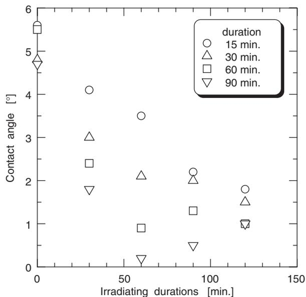
Fig. 5. Changes in contact angles of water with the duration of ultraviolet (UV) irradiation.
