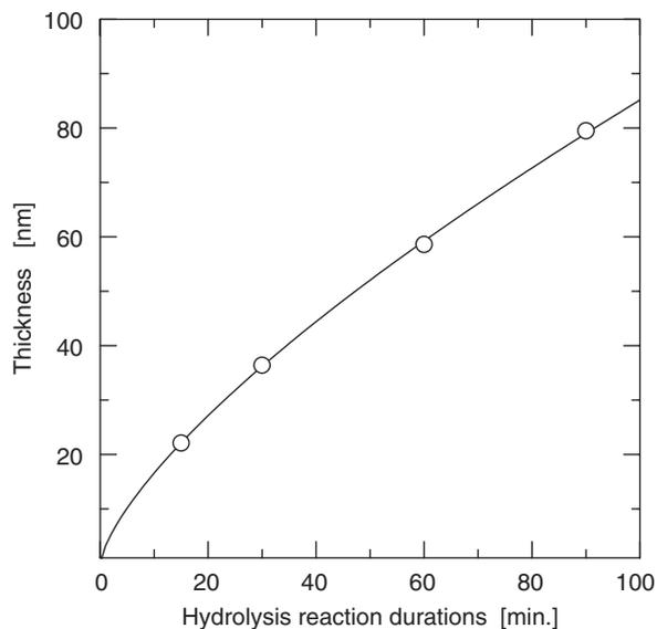
Fig. 4. Thickness of anatase titanium dioxide thin films on slide glass surfaces.
