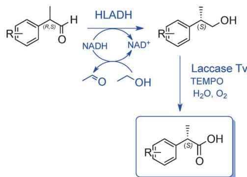
**Figure 2.** Chemoenzymatic route to enantiomerically pure arylpropionic acids. HLADH = horse liver alcohol dehydrogenase, NADH/NAD<sup>+</sup> = nicotinamide adenine dinucleotide redox couple.
