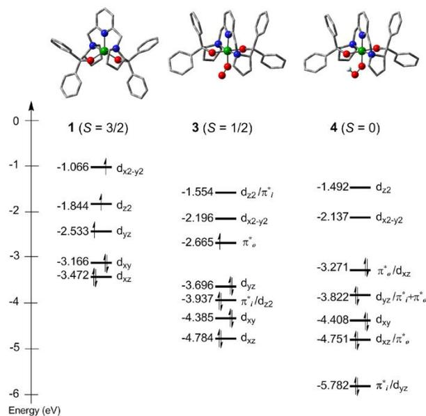
**Figure 5.** The represented d-manifold splitting patterns and  $\text{O}_2^-/\text{HOO}^- \pi^*$  orbitals of DFT-optimized **1**, **3**, and **4** where the orbital energies are obtained from their corresponding  $\beta$ -spin orbitals, respectively. The notions *i* and *o* of  $\text{O}_2^-/\text{HOO}^- \pi^*$  orbitals are referred to “in-plane” and “out-of-plane”, respectively. The planes for the notations are defined as Co-O-O for **3** and O-O-H for **4**.
