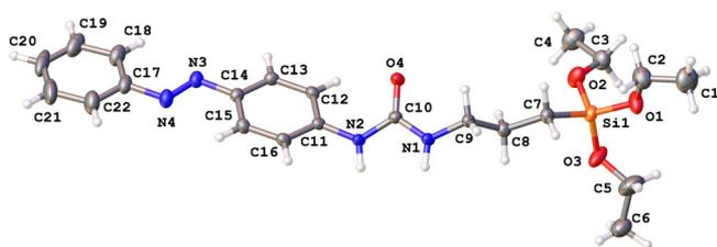
**Figure 1.** Molecular structure of **2** (probability level of displacement ellipsoids at 50%).
