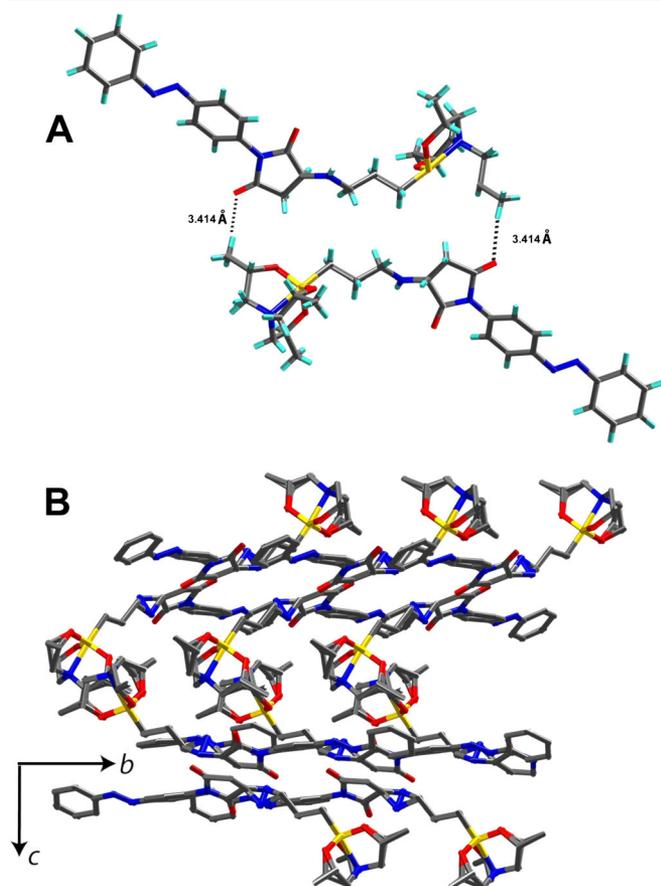
**Figure 4.** Molecular structure of **9** with packing and interactions. (A) Pair of molecules joined by non-classical interactions of methyl C9 and O5 with bond length of 2.416 Å. (B) Lattice arrangement of three-dimensional pattern along *a*-axis showing an alternate layer-type arrangement of silatrane moiety and the rest of the alkyl chain.
