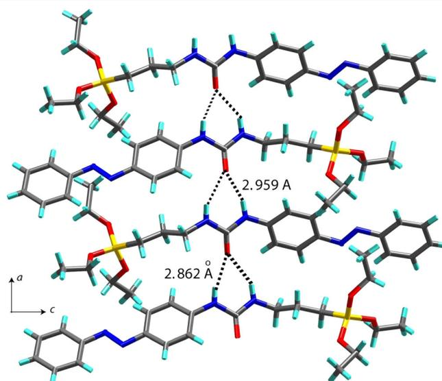
**Figure 2.** Molecular lattice arrangement for compound **2** along  $b$ -axis. Molecules are packed via weak hydrogen-bonding interactions between adjacent urea moieties of 2.959(2) and 2.862(2) Å.
