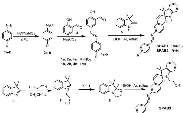
**Figure 3.** Synthesis routes of SPAB derivatives
