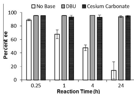
**Figure 1.** Effect of reaction time and added base on the observed ee of (*R*)-**3** with ligand **4** (PHOX). Each time point is the average of 4–7 individual reaction trials with error bars showing  $\pm 1$  standard deviation.
