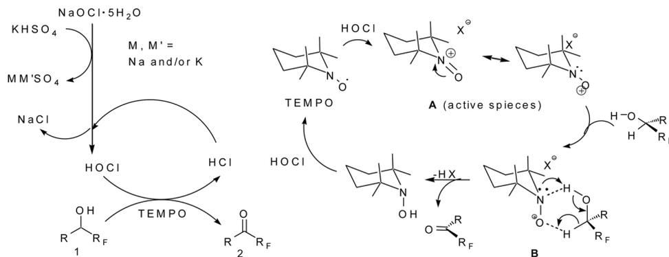
Scheme 4. Plausible reaction mechanism.
