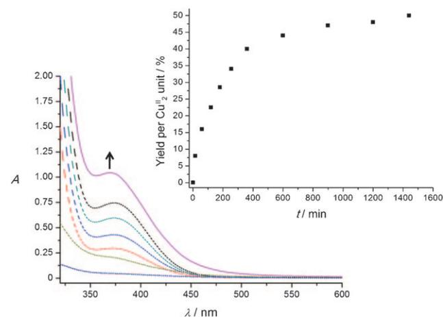
**Figure 2.** UV/Vis spectroscopic monitoring of the formation of 1,3-bis(*m*-hydroxybenzylidene)acetone after oxygenation and derivatization (see text for additional information) of a 12.5 mM solution of **1** during the first 4 h (dotted lines; navy blue: *t* = 0 min, dark yellow: *t* = 30 min, red: *t* = 1 h, blue: *t* = 2 h, cyan: *t* = 3 h, black: *t* = 4 h) and after one day (solid line; magenta); *l* = 1 cm. Inset: Yield per dicopper unit as a function of time.
