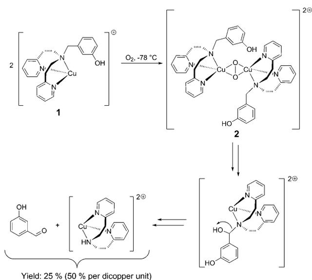
**Scheme 2.** Reaction sequence leading to the formation of *m*-hydroxybenzaldehyde. Intermediate **2** is generated upon reaction of **1** with dioxygen at low temperature. The benzylic ligand hydroxylation with subsequent N-dealkylation was observed instead of the intended aromatic hydroxylation. Counterions and the equilibrium of the Cu<sup>II</sup><sub>2</sub> μ-η<sup>2</sup>:η<sup>2</sup>-peroxo species with its bis(μ-oxo) dicopper(III) analogue in compound **2** are neglected.
