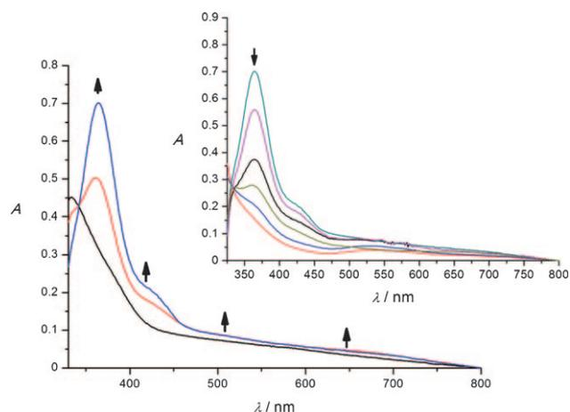
**Figure 1.** UV/Vis spectra of a 1 mM solution of the precursor complex **1** in acetone under argon atmosphere (black) and its oxygenation product **2** after reaction of **1** with O<sub>2</sub> at -78 °C for 3 min (red) and 5 min (blue); *l* = 0.1 cm. Inset: Decomposition of **2** beginning after 8 min of oxygenation and measured in 30 min intervals.
