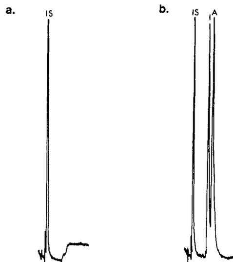
**Figure 1**—Chromatograms of (a) blank with internal standard and (b) acitretin and isoacitretin at 1000 pmol/200  $\mu$ L. Key: (IS) internal standard, etretinate; (I) isoacitretin; (A) acitretin.
