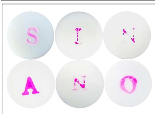
Fig. 6 Specimens of water-carved urethane-bridged silica aerogels
