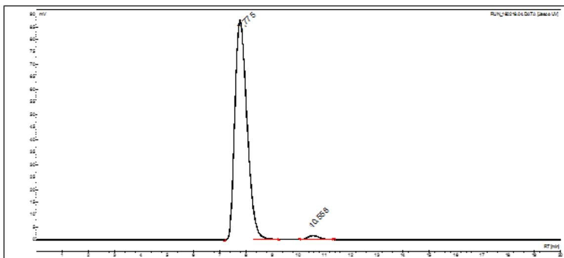
Figure 5. HPLC chromatogram (UV-signal, 254 nm) of reference compound **1b**; analytical column, 50% MeCN/50% 0.1% TFA (v/v), flow 1 mL/min
