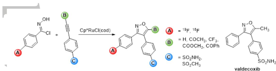
Scheme 1.  $^{18}/^{19}\text{F}$ -labelled isoxazoles by Ru-promoted 1,3-dipolar cycloaddition of  $^{18}/^{19}\text{F}$ -labelled nitrile oxides with alkynes.
