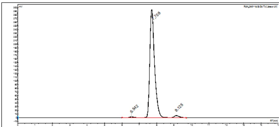
Figure 3. HPLC chromatogram (UV-signal, 254 nm) of reference compound **1e**; semi-preparative column, 50% MeCN/50% 0.1% TFA (v/v), flow 5 mL/min
