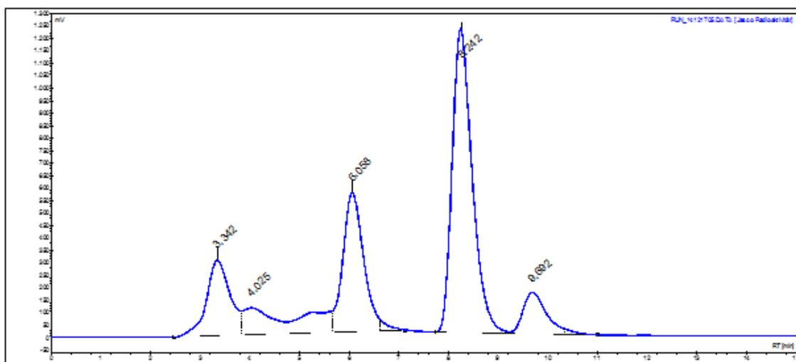
Figure 2. Radio HPLC chromatogram of reaction mixture of Ru-promoted 1,3-dipolar cycloaddition of  $^{18}\text{F}$ FBIC with methyl 3-(4-(methylsulfonyl)phenyl)prop-2-ynoate, 10 min, 45°C; semi-preparative column, 50% MeCN/50% 0.1% TFA (v/v), flow 5 mL/min
