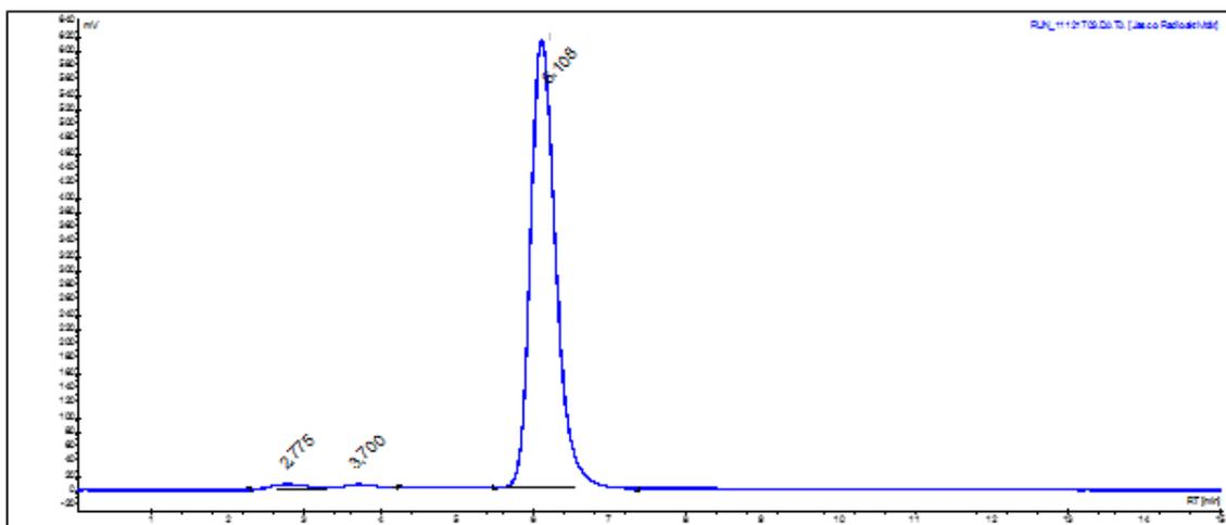
Figure 1. Radio-HPLC chromatogram of purified  $^{18}\text{F}$ FBIC; semi-preparative column, 50% MeCN/50% 0.1% TFA (v/v), flow 5 mL/min
