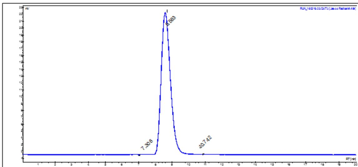
Figure 4. Radio HPLC chromatogram of purified [ $^{18}\text{F}$ ]**1b**; analytical column, 50% MeCN/50% 0.1% TFA (v/v), flow 1 mL/min
