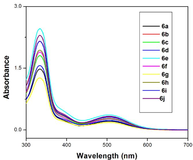
**Fig. 3.** UV-Vis spectra of triazole 6(a-j) in acetonitrile at room temperature.
