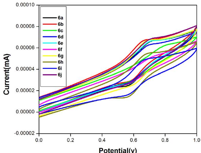
**Fig. 4.** Electrochemical oxidative potential curves of 6(a-j) in acetonitrile at room temperature. All the compounds 6(a-j) in  $\text{CH}_3\text{CN}$  with TBAP (supporting electrolyte) at  $25^\circ\text{C}$  at a scan rate of  $100 \text{ mV s}^{-1}$ .
