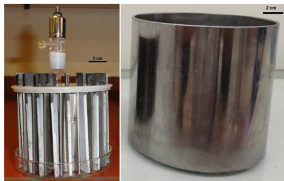
Figure 8. Images of employed electrochemical cell with 260 cm 2 geometric area of working electrode; inner (a) and outer (b) parts
