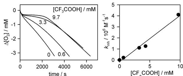
Fig. 1 (A) Oxygen uptake kinetics during the autoxidation of 4.3 M styrene in MeCN initiated by 0.05 M AIBN at 303 K inhibited by 12.5  $\mu\text{M}$  TEMPO with variable amounts of trifluoroacetic acid, and (B) dependence of the measured inhibition rate constant ( $k_{\text{inh}}$ ) on the concentration of acid.
