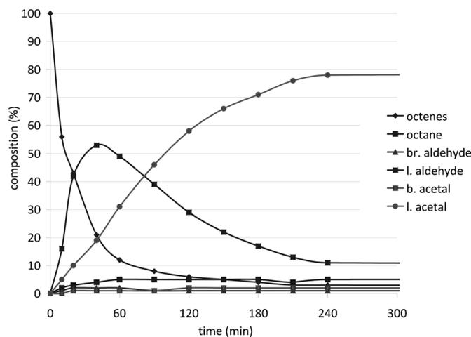
**Figure 3.** Reaction profile of the 1,1-dimethoxynonane formation. 1-octene (10 mmol),  $[\text{Rh}(\text{cod})_2\text{BF}_4]$  (S/Rh=400), Xantphos (L/Rh=3), MeOH (200 mmol),  $\text{CO}/\text{H}_2$  (30 bar, 1:2),  $110^\circ\text{C}$ .
