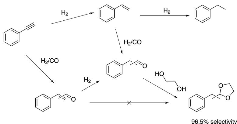
**Scheme 3.** Reaction with phenylacetylene.
