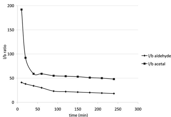
**Figure 4.** Evolution of l/b ratio in time. 1-octene (10 mmol),  $[\text{Rh}(\text{cod})_2\text{BF}_4]$  (S/Rh=400), Xantphos (L/Rh=3), MeOH (200 mmol),  $\text{CO}/\text{H}_2$  (30 bar, 1:2),  $110^\circ\text{C}$ .
