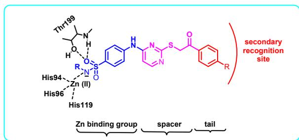
**Figure 3.** The design strategy for the novel pyrimidine-sulfonamide conjugates as hCA inhibitors
