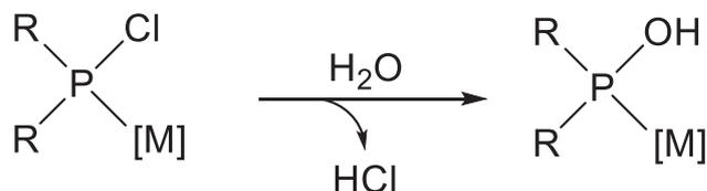
**Scheme 3:** Alternative procedure to generate complexes with  $\text{PR}_2\text{OH}$  ligands.
