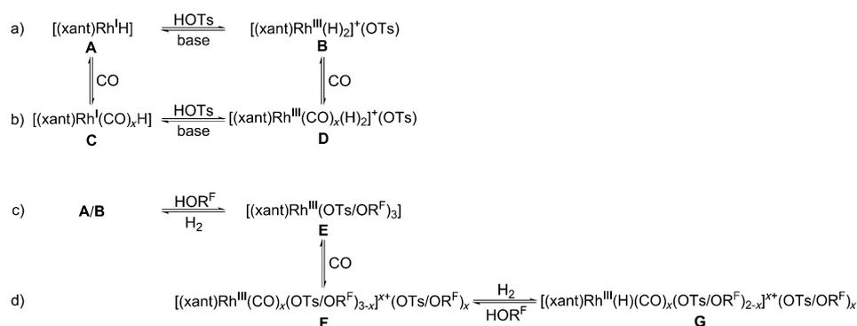
**Scheme 5.** Generation of various hydrogenation catalysts under reductive amidation conditions (xant = xantphos): a) in pure diglyme with a H<sub>2</sub> atmosphere; b) in diglyme with a H<sub>2</sub>/CO atmosphere; c) in HOR<sup>F</sup>/diglyme with a H<sub>2</sub> atmosphere; and d) in HOR<sup>F</sup>/diglyme with a H<sub>2</sub>/CO atmosphere.
