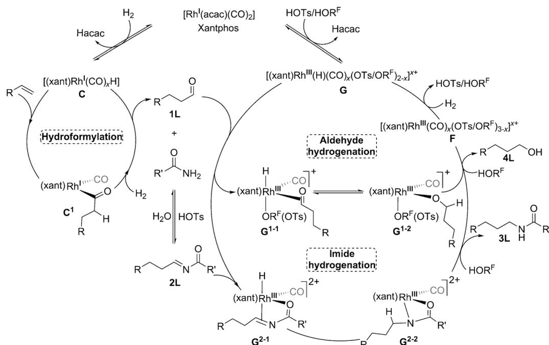
**Scheme 6.** Proposed overall mechanism for the hydroamidomethylation of 1-alkenes.
