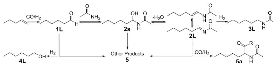
**Scheme 4.** Catalytic hydroamidomethylation of 1-pentene: a one-pot synthesis of **3L** through the formation of **1L** and intermediate **2L**; **4L** and heavy-ends **5** are undesired byproducts (for clarity only the linear products are depicted). R in **5a** can be H (CHO) or OH (COOH).
