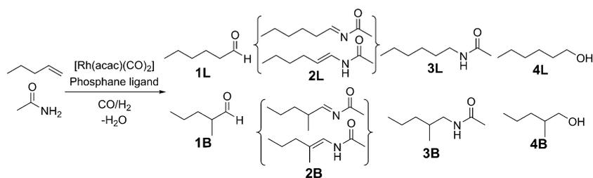
**Scheme 3.** Hydroamidomethylation of 1-pentene with acetamide: observed intermediates, products, and undesired byproducts.
