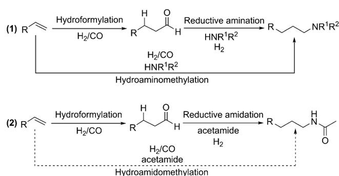
**Scheme 1.** Hydroaminomethylation versus the hydroamidomethylation reaction.
