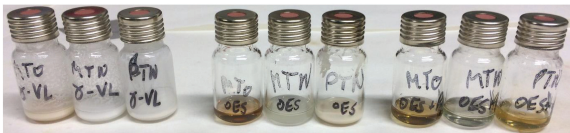
Fig. 7 Solubility tests of polyaramid oligomers. Left: solubility in only GVL, centre: solubility in [C_8MIm][Cl]/GVL OES with x_{IL} = 0.043 , right: OES also containing [2-Me-HPyr][Cl] . Solubility of the oligomers increases from left to right.
