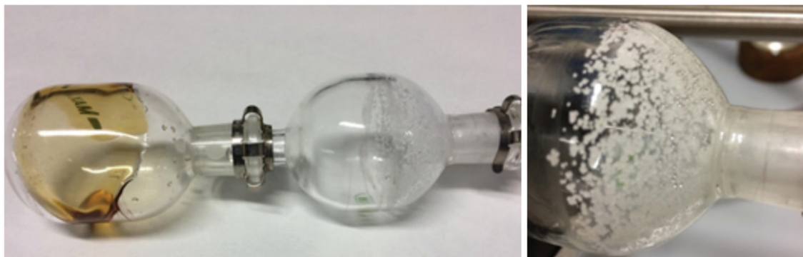
Fig. 11 Separation of [\text{C}_8\text{MIm}][\text{Cl}] and [\text{2-Me-HPyr}][\text{Cl}] via short path distillation in a Kugelrohr apparatus.
