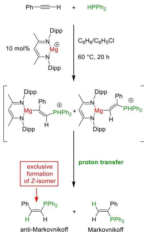
**Scheme 2.** Reaction of  $\text{PhC}\equiv\text{CH}$  with  $\text{HPPH}_2$  catalyzed by  $\left[ \left( \text{BDI} \right) \text{Mg}^+ \cdot \text{C}_6\text{D}_6 \right] \left[ \text{B}(\text{C}_6\text{F}_5)_4^- \right]$ . The exclusive formation of the Z-isomer for the anti-Markovnikoff product confirms rear-side attack of the alkyne by  $\text{HPPH}_2$ .
