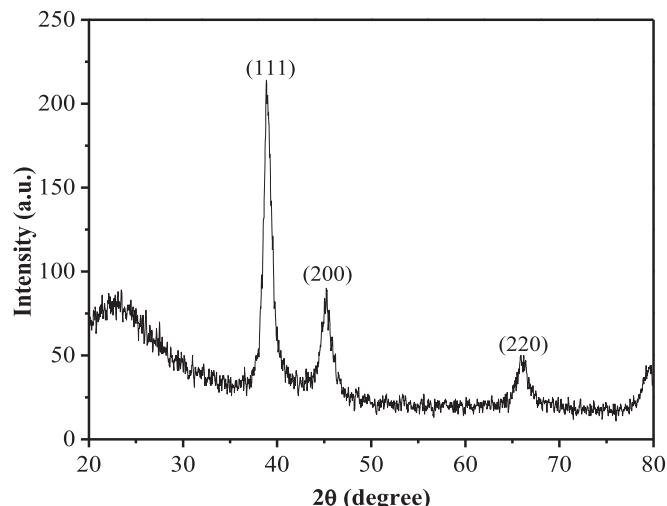
Fig. 5. Wide angle XRD patterns of MCM-41-3N-Pd(0).
