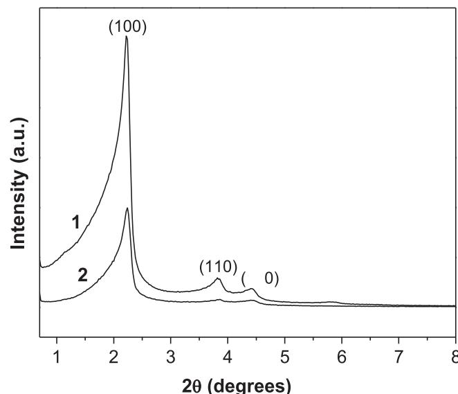
Fig. 1. Small angle XRD patterns of MCM-41 (1) and MCM-41-3N-Pd(0) (2).
