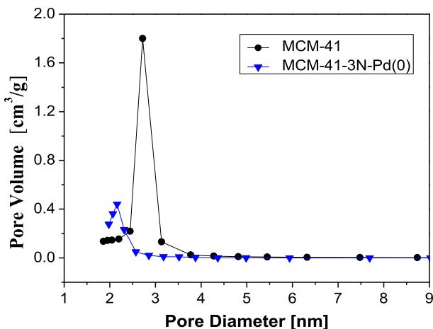
Fig. 3. Pore size distributions of MCM-41 and MCM-41-3N-Pd(0).
