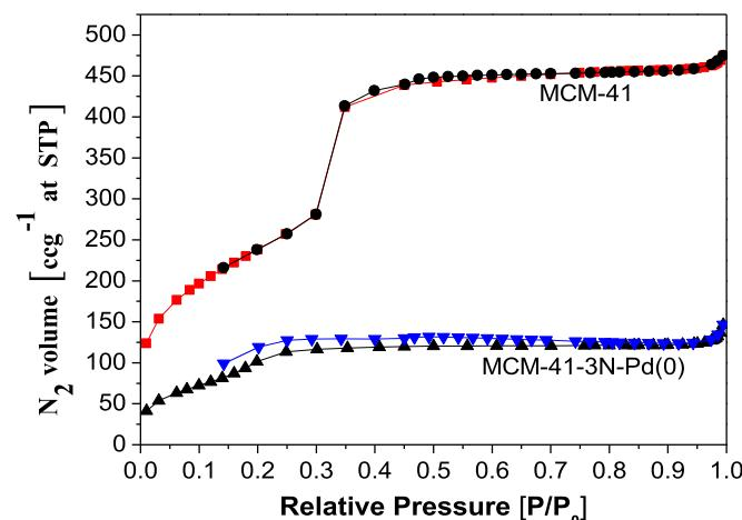
Fig. 2.  $\text{N}_2$  adsorption/desorption isotherms of MCM-41 and MCM-41-3N-Pd(0).
