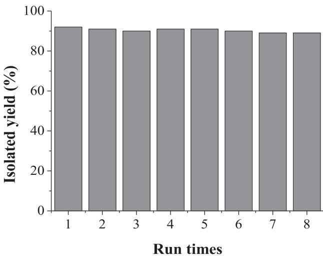
Fig. 6. Recycle of MCM-41-3N-Pd(0) catalyst.
