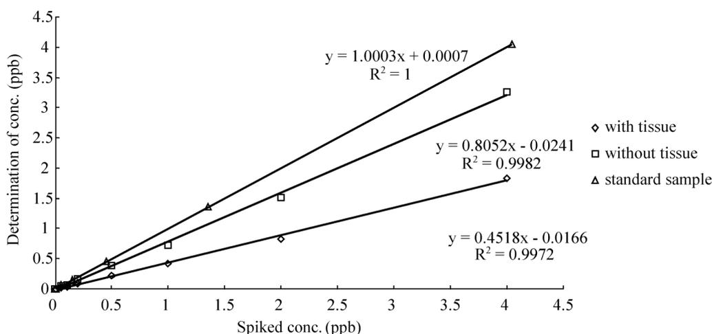
Fig. 5. Calibration curves for: (a) spiked specific concentrations in samples with fish tissue, (b) spiked specific concentrations in samples without fish tissue, (c) standard solutions in the ELISA kits.
