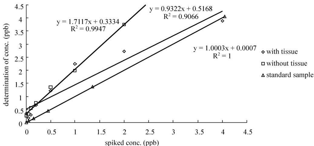
Fig. 6. Calibration curves for: (a) spiked specific concentrations in samples with fish tissue, (b) spiked specific concentrations in samples without fish tissue, (c) standard solutions in the ELISA kits.
