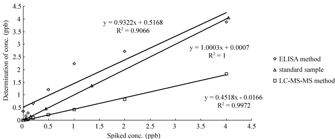
Fig. 7. Comparison of calibration curves for ELISA method, standard sample and LC-MS/MS method.
