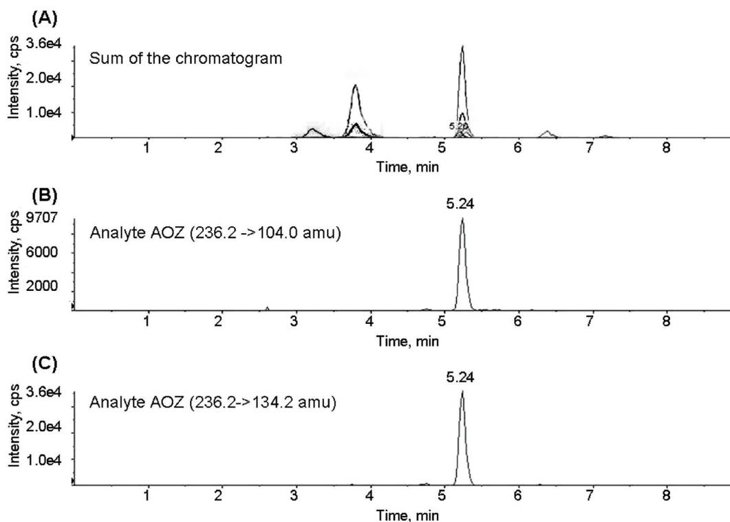
Fig. 4. LC-MS/MS chromatograms (MRM) of spiked 5.0 ng/g AOZ in *Tilapia* fish tissue. (A) sum of the chromatogram, (B) confirmation of analyte AOZ (236.2  $\rightarrow$  104.0 amu), (C) quantification of analyte AOZ (236.2  $\rightarrow$  134.2 amu).
