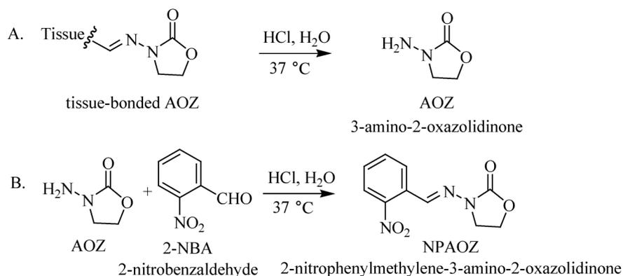
Fig. 1. The structures of tissue-bonded AOZ (3-amino-2-oxazolidinone), released type of AOZ, derivative reagent 2-NBA (2-nitrobenzaldehyde) and target derivative NPAOZ (2-nitrophenylmethylene-3-amino-2-oxazolidinone).
