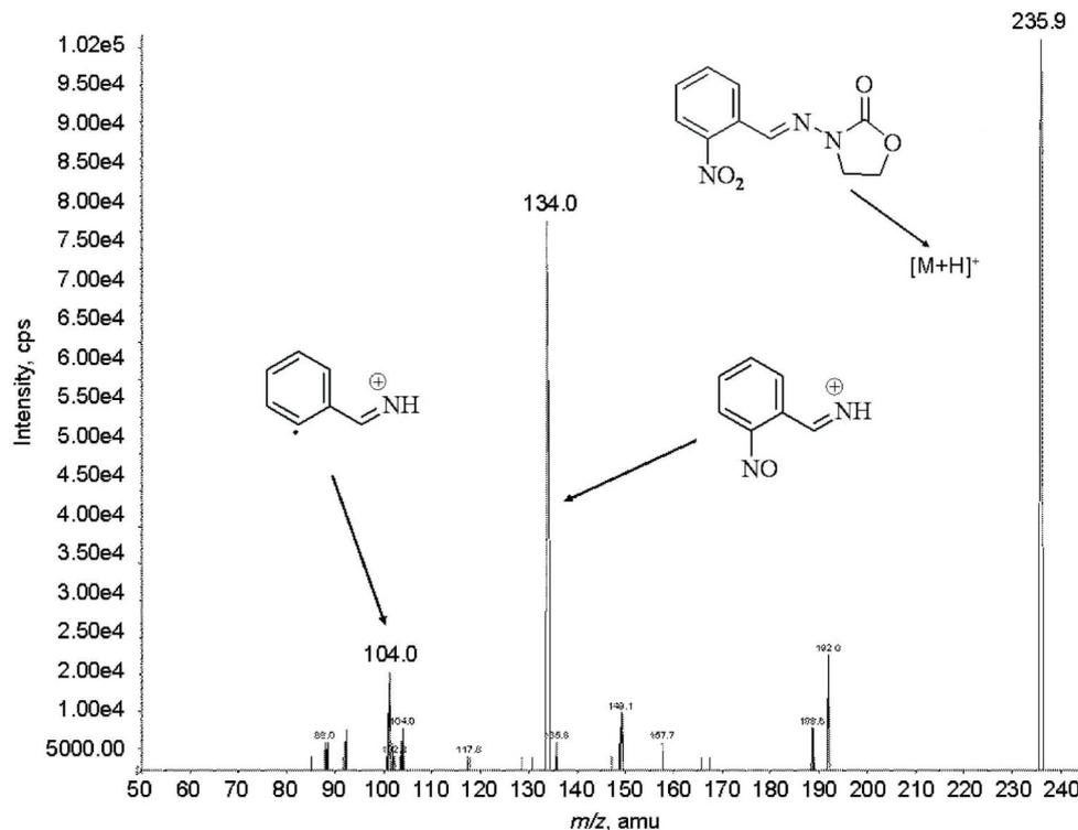
Fig. 2. Mass spectrum of NPAOZ and its typical fragmentation pattern.
