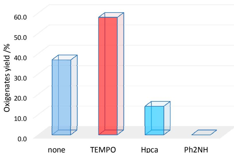
**Figure 4** - Effect of different additives on the yield of cyclohexanol and cyclohexanone obtained by microwave-assisted neat oxidation of cyclohexane with THBP, catalysed by **2** (0.1% molar vs. substrate).
