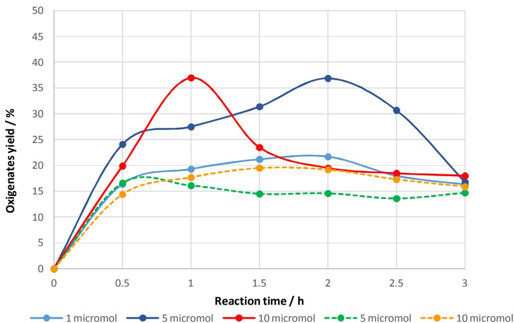
**Figure 6** - Effect of the reaction time and catalyst (— **2** or ---- **1**) amount on the yield of cyclohexanol and cyclohexanone obtained by additive-free microwave-assisted neat oxidation of cyclohexane with THBP.
