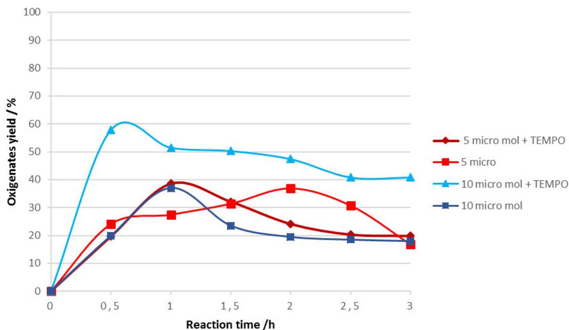
**Figure 5** - Effect of the reaction time, catalyst **2** amount and TEMPO additive on the yield of cyclohexanol and cyclohexanone obtained by microwave-assisted neat oxidation of cyclohexane with THBP.
