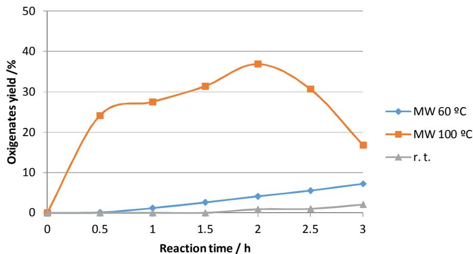
**Figure 7.** Effect of reaction temperature on the yield of cyclohexanol and cyclohexanone obtained by the additive-free neat oxidation of cyclohexane with THBP, catalysed by **2** (0.1% molar vs. substrate).
