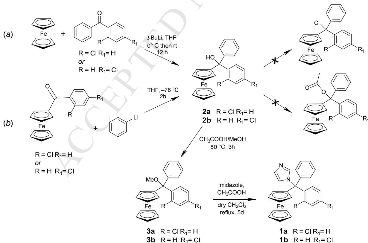
**Scheme 4.** Synthesis of the ferrocenyl analogues of clotrimazole
