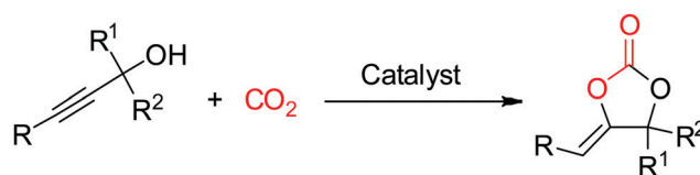
Scheme 1 Coupling of propargyl alcohol with CO 2 affording \alpha -alkylidene cyclic carbonate.
