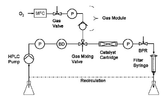
Scheme 1. Process schematic of the reactor (H-Cube Pro with Gas Module, Thales Nanotechnology Inc., Hungary). 24 P=pressure sensor, BD=bubble detector, MFC=mass flow controller, BPR=back-pressure regulator.
