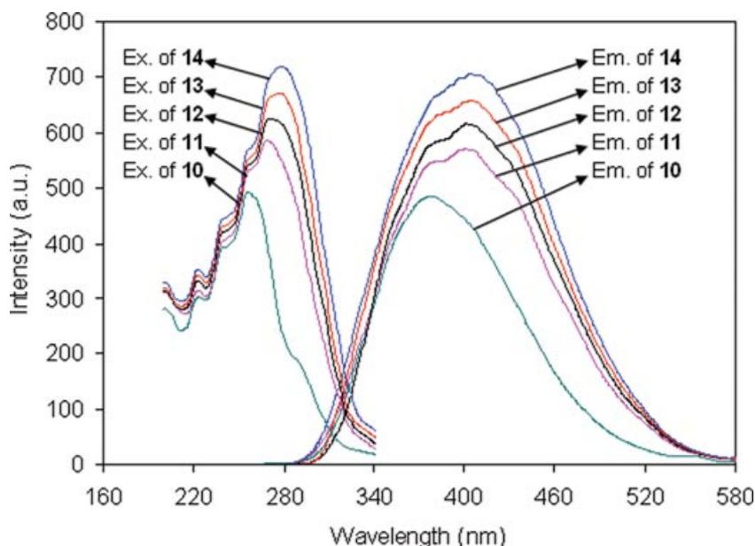
**FIGURE 3** Photoluminescence spectra of 5-amino-1,3,4-thiadiazole-2-sulfonamide (**10**) and 5-(4-alkyl-1-naphthoylamino)-1,3,4-thiadiazole-2-sulfonamides **11–14** in  $\text{CHCl}_3$ ; samples were excited at 261 nm.
