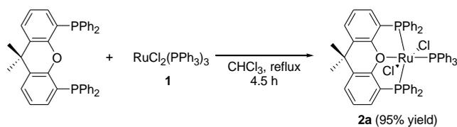
**Scheme 1** Preparation of  $\text{RuCl}_2(\text{xantphos})(\text{PPh}_3)$  (**2a**).
