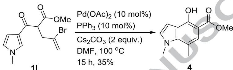
**Scheme 2.** Synthesis of indole-5-carboxylate **4** via palladium catalyzed C–H alkenylation of **1l**.
