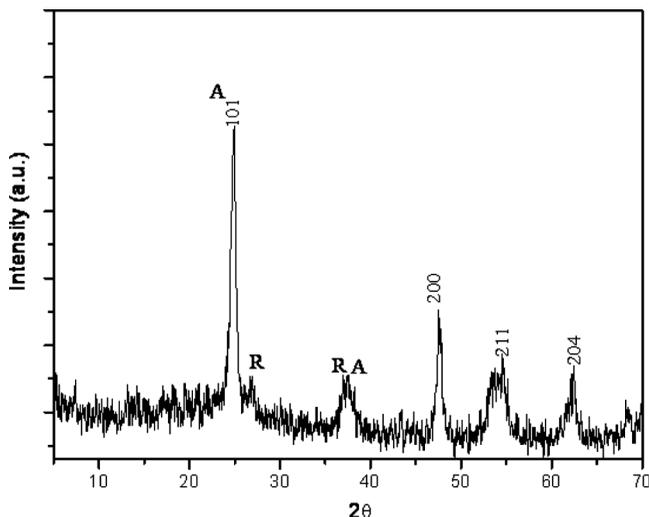
Figure 1. Powder XRD pattern of nanocrystalline titanium(IV) oxide.
