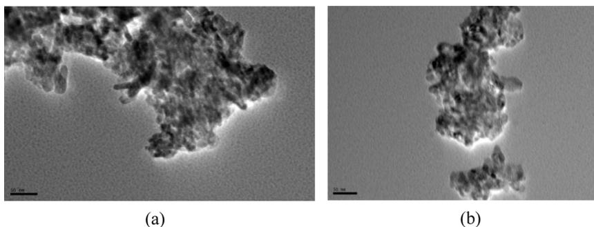
**Figure 2.** (a) TEM images of fresh nanoparticles; (b) TEM images of recycled nanoparticles.
