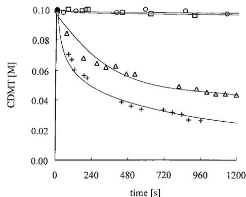
**Figure 1.** Rate of activation of trimethylacetic acid in acetonitrile-*d*<sub>3</sub> solution by means of **1** relative to the structure of the tertiary amine: for *N*-methylmorpholine (—+—+—); *N,N*-tetramethylethylenediamine (—Δ—Δ—); triethylamine (—○—○—); *N,N*-dimethylaniline (—□—□—).
