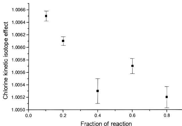
**Figure 5.** Experimental chlorine isotope effect (changes with reaction progress).
