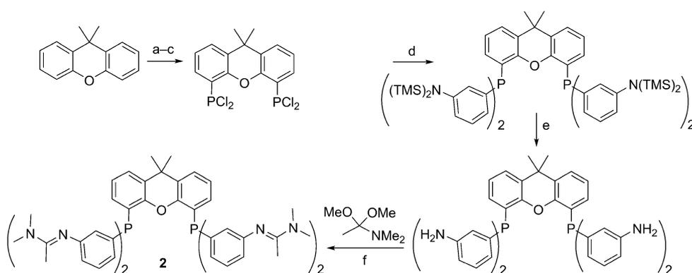
**Scheme 3.** Synthesis of **2**: a) THF, BuLi, -78 °C to RT, 24 h; b) (NEt<sub>2</sub>)<sub>2</sub>PdCl, -78 °C to RT, 24 h; c) HCl<sub>(g)</sub>, 0 °C, 15 min; d) 3-[bis(trimethylsilyl)amino]phenylmagnesium chloride, -78 °C to RT 12 h, 55 °C, 12 h; e) MeOH, reflux, overnight; f) Microwave, 160 °C, 1 h. TMS = trimethylsilyl.
