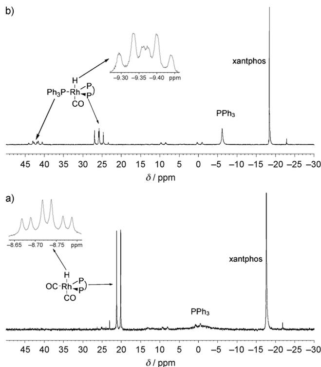
**Figure 2.** <sup>31</sup>P{<sup>1</sup>H} NMR and the hydride region of the <sup>1</sup>H NMR spectra (inset) that were measured at room temperature for a mixture of [Rh(acac)(CO)<sub>2</sub>], PPh<sub>3</sub>, and xantphos (1:2:2) a) Under CO/H<sub>2</sub> (1:1, 15 bar) and b) The solution from a) after bubbling CO<sub>2</sub> through the solution for 15 min.
