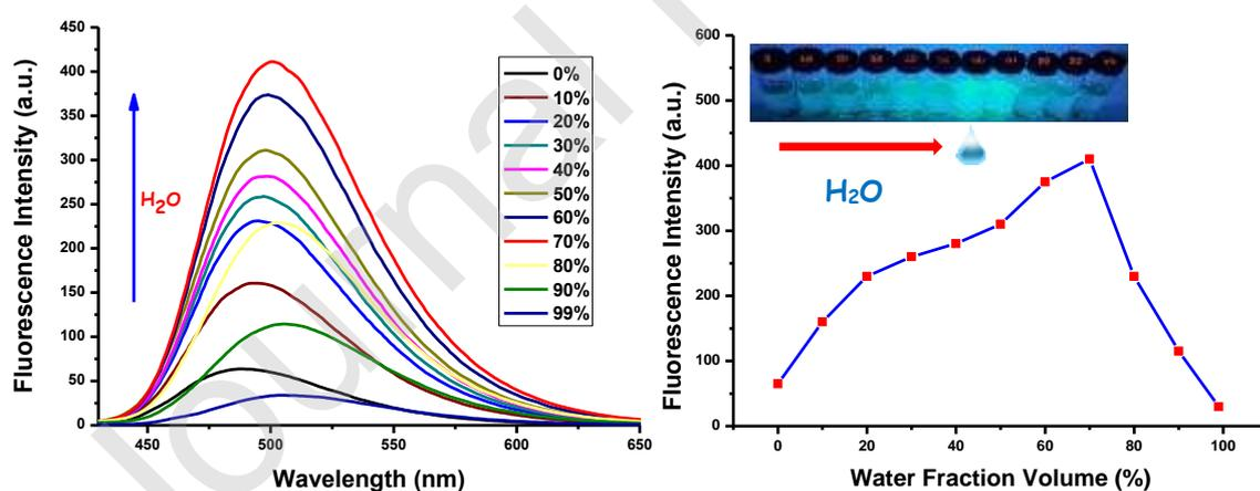
**Fig. 1.** Fluorescence intensity change spectrum of **ANT-Fe** (10  $\mu$ M) in CH<sub>3</sub>CN with increasing volume of water percentages from 0% to 99%.
