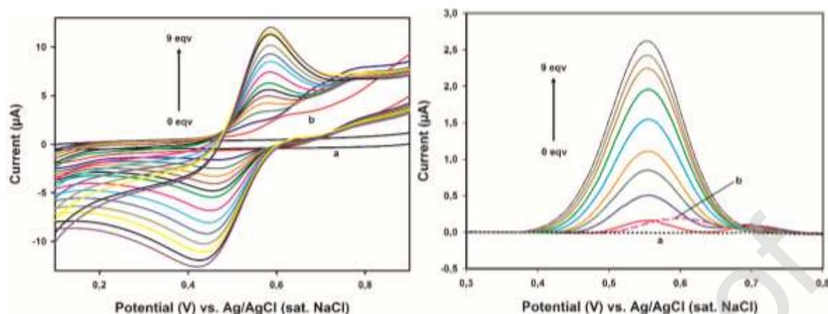
**Fig. 7.** CV and DPV titrations of the **ANT-Fe** with addition of different concentrations of  $\text{Cu}^{2+}$  (0 – 9 equiv.) (a): Acetonitrile solution (b): 200  $\mu\text{M}$  **ANT-Fe** only (in 4:1  $\text{CH}_3\text{CN}$  : HEPES (v/v) solution at pH = 7.0)
