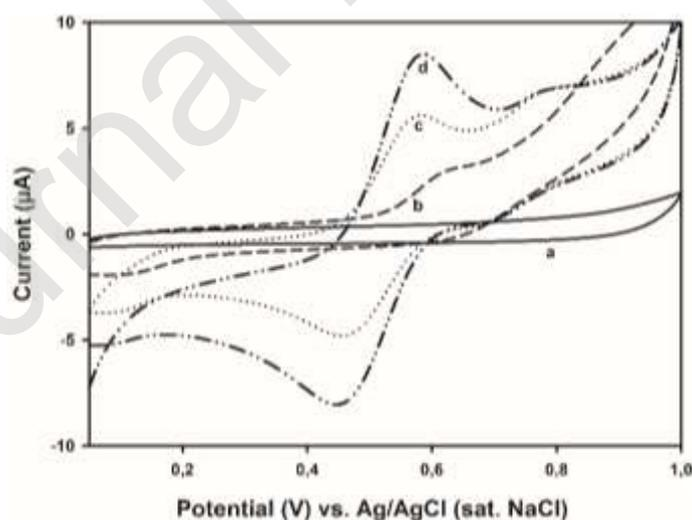
**Fig. 6.** CV results of (a) acetonitrile, (b) 200  $\mu\text{M}$  **ANT-Fe** only (c) **ANT-Fe** and 2.5 equivalent  $\text{Cu}^{2+}$  (d) pure ferrocenecarboxaldehyde only (in 4:1  $\text{CH}_3\text{CN}$  : HEPES (v/v) solution at pH = 7.0)
