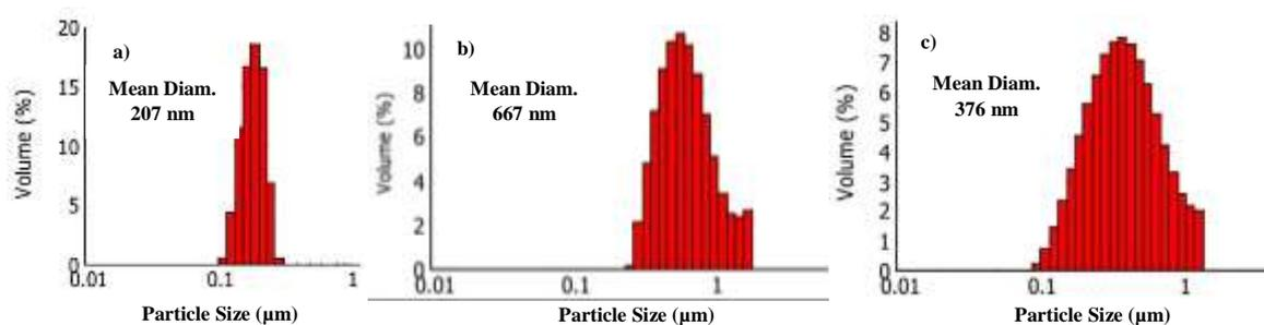
**Fig. 2.** The particle size distribution of **ANT-Fe** (10  $\mu\text{M}$ ) in mixed aqueous solutions ( $\text{CH}_3\text{CN}/\text{H}_2\text{O}$ ) of (a) 40%, (b) 70% and (c) 90% volume of water content determined by DLS measurements
