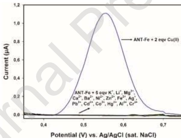
**Fig. 8.** DPV measurements of **ANT-Fe** and  $\text{Cu}^{2+}$  (2.0 equiv.) and other cations (2.0 equiv.) in 4:1  $\text{CH}_3\text{CN}$  : HEPES (v/v) solution at pH = 7.0
