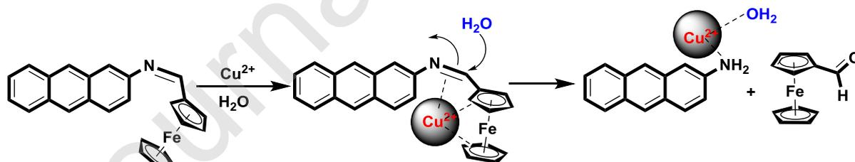
**Scheme 2.** Proposed mechanism for the detection of  $\text{Cu}^{2+}$  ions
