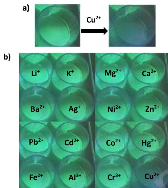
**Fig. 9.** (a) Fluorescence images of **ANT-Fe** adsorbed on test paper before and after addition of  $\text{Cu}^{2+}$  ( $50 \mu\text{M}$ ) under UV light at 366 nm (b) Detection of different metal ions ( $100 \mu\text{M}$ ) with **ANT-Fe** on TLC test paper fluorescence images under UV light at 366 nm (All images were recorded after 5 min).
