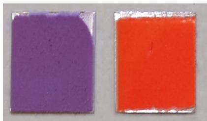
**Figure 4.** Image of the TLC plates with absorbed **3PEG-Ru-CH=CH-per<sup>lm</sup>** (left) and **3PEG-Ru-py-per<sup>lm</sup>** (right).
