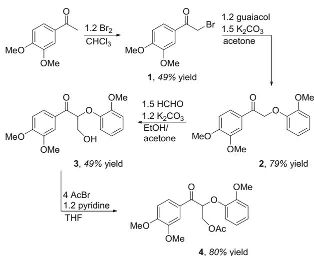
**Scheme 1** Synthesis of the γ-acetylated β-O-4 ketone dimer lignin model compound **4**
