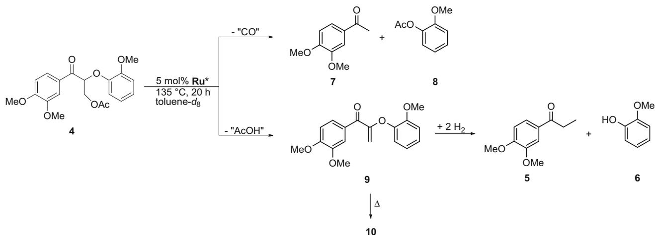
**Scheme 3** Proposed mechanistic pathways for hydrogenolysis of **4**
