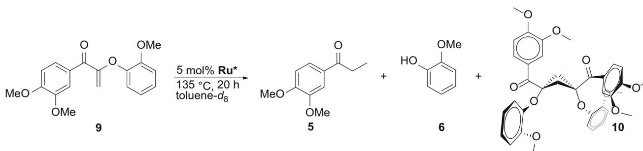
**Scheme 5** Products of the catalytic hydrogenolysis of **9**
