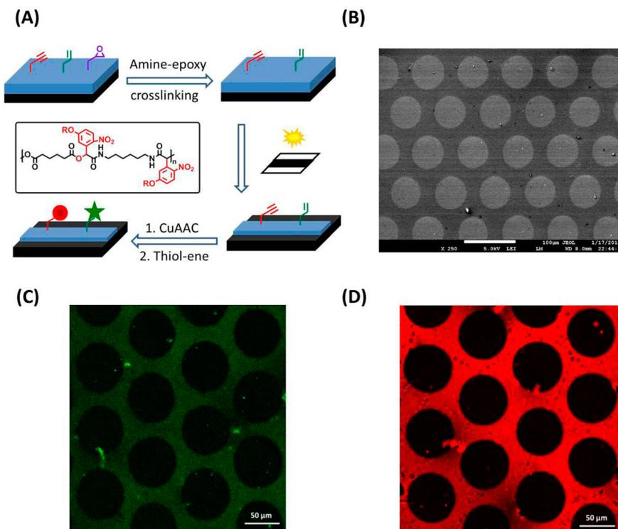
**Figure 5.** (A) Schematic representation of the process for generation of multifunctional pattern on silicon wafer using **P4** as a photoresist; (B) SEM image of the patterned film (scale bar = 100  $\mu\text{m}$ ); confocal fluorescence images of the patterned film functionalized with Azido-FITC (C) and rhodamine dye (D) (scale bar = 50  $\mu\text{m}$ ).
