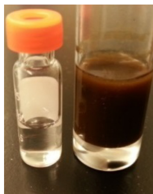
Fig. 4. Reusability test of PPPd in Suzuki-Miyaura coupling reactions (left) and a typical reaction mixture as well as the liquid phase after filtration (right).
