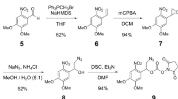
**Scheme 2.** Four-step synthesis of the photocleavable linker **9**. NaHMDS = sodium bis(trimethylsilyl)amide.
