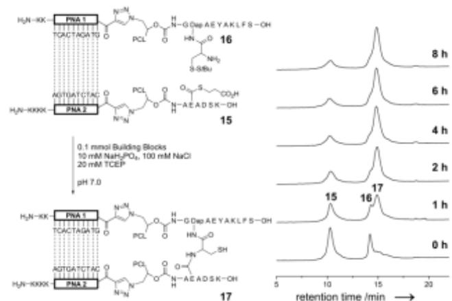
**Scheme 4.** Template-directed native chemical ligation between thioester hybrid **15** and cysteine hybrid **16**. HPLC chromatograms after 0, 1, 2, 4, 6, and 8 h indicate consumption of hybrids **15** and **16** and formation of ligation product **17**. Conversion of thioester hybrid **15**: 38% (1 h), 53% (2 h), 62% (4 h), 64% (6 h), 67% (8 h).
