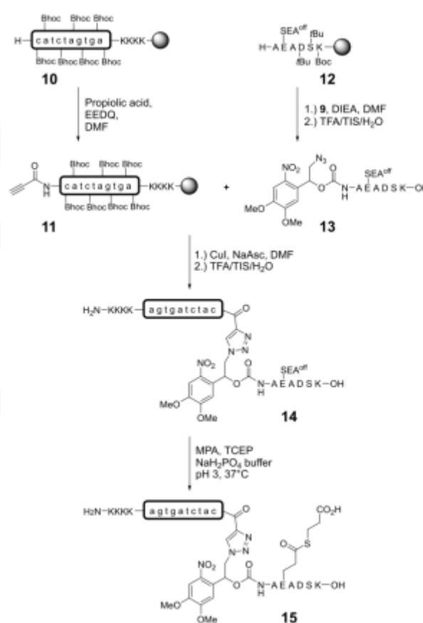
**Scheme 3.** Convergent strategy for the peptide/PNA hybrid synthesis. Modification of the PNA strand (**11**), attachment of the caging group (**13**) and subsequent PNA/peptide synthesis by CuAAC (**14**) are equal for all hybrids. For thioester hybrids an additional transthioesterification step is necessary.
