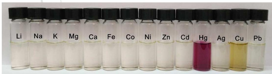
**Fig. 6.** Visual color changes of chemosensor **2a** upon addition of various metal ions (1 equiv.) in CH<sub>3</sub>CN (1×10<sup>-4</sup> M).
