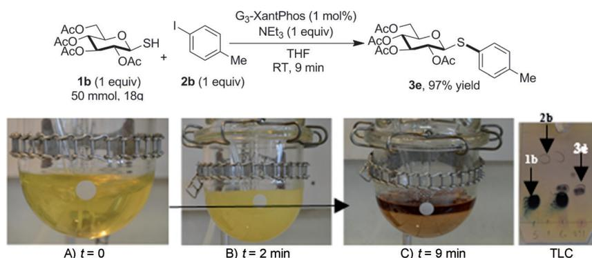
**Figure 1.** Multigram-scale coupling of 1-thio-β-D-glucopyranose **1b** with 4-iodotoluene **2b** at RT in a reactor.
