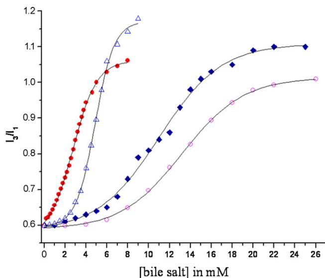
Fig. 2. The ratio of vibronic bands ( $I_3/I_1$ ) of pyrene fluorescence as a function of bile salt concentration at pH 9.0 (TRIS buffer) at 25°C; (●) PCA; (△) DCA; (◆) 16-EPCA; (○) CA.
