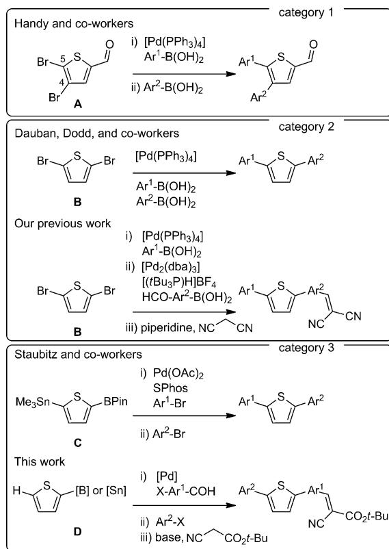
**Scheme 1.** One-pot, multi-component coupling approaches for the synthesis of oligo-thiophenes. dba = dibenzylideneacetone; Pin = pinacol; SPhos: 2-di-cyclohexylphosphino-2',6'-dimethoxybiphenyl.
