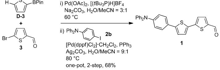
**Scheme 3.** Examination of one-pot, three-component coupling reactions for the synthesis of **1**.
