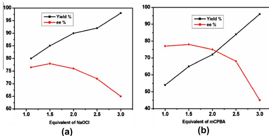
**Figure 3.** Effect of the amount of (a) NaOCl and (b) *m*CPBA on the enantioselective epoxidation of 2,2-dimethylchromene (4 mol % of **20** was used in both cases).
