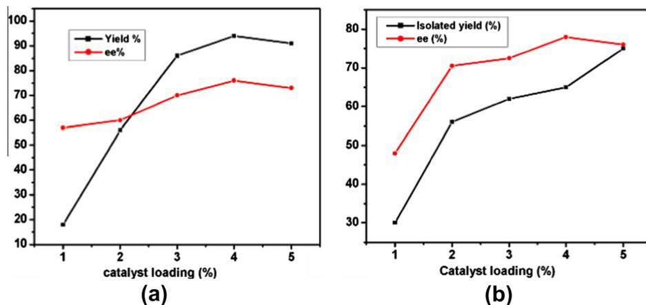
**Figure 4.** Effect of catalyst loading on the enantioselective epoxidation of 2,2-dimethylchromene with (a) NaOCl (2 equiv) and (b) *m*CPBA (1.5 equiv) as terminal oxidant.
