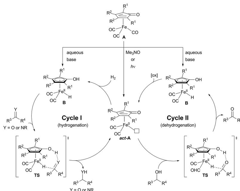
Scheme 1. Catalytic pathways of (i) hydrogenation of C=O and C=N double bonds (Cycle I) and (ii) Oppenauer-type alcohol oxidation (Cycle II) catalyzed by cyclopentadienone complexes **act-A**.
