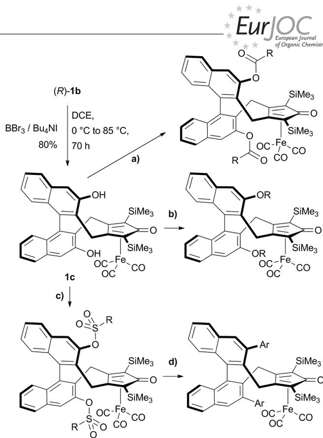
Scheme 5. General synthetic strategy for the preparation of 3,3'-substituted (cyclopentadienone)iron complexes **I**: (a) esterification, (b) etherification, (c) sulfonylation, and (d) cross-coupling.
