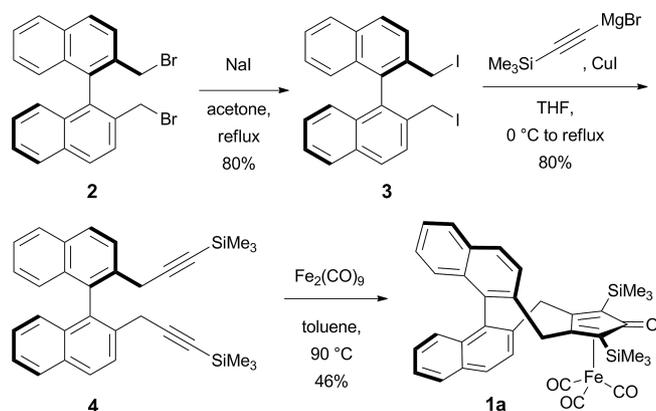
Scheme 2. Synthesis of the precatalyst (*R*)-**1a**.<sup>[24]</sup>
