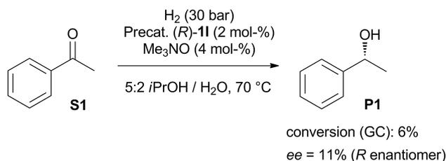
Scheme 11. Test of precatalyst (*R*)-**11** in the AH of acetophenone under the optimized conditions [substrate/(*R*)-**11**/ $\text{Me}_3\text{NO}$  100:2:4,  $P_{\text{H}_2}$  = 30 bar, solvent = 5:2 *i*PrOH/ $\text{H}_2\text{O}$ ,  $c_0$ (substrate) = 1.43 M,  $T$  = 70 °C, reaction time: 18 h].
