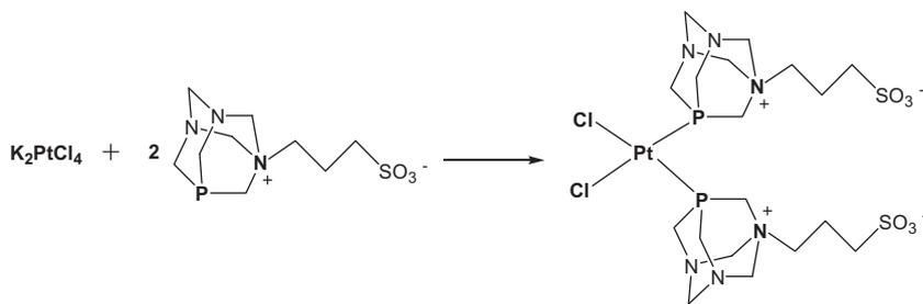
**Scheme 3.** Synthesis of the Pt complex  $\text{cis-}[\text{PtCl}_2(\text{PTA}^+\text{C}_3\text{H}_6\text{SO}_3^-)]_2$ , **5**.
