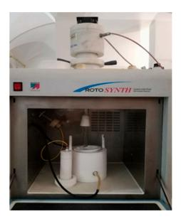
Figure 8. Combined MW/US device.
